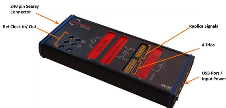
Figure 16 Illustration of the SV3C CPTX C-PHY Generator connectors.
